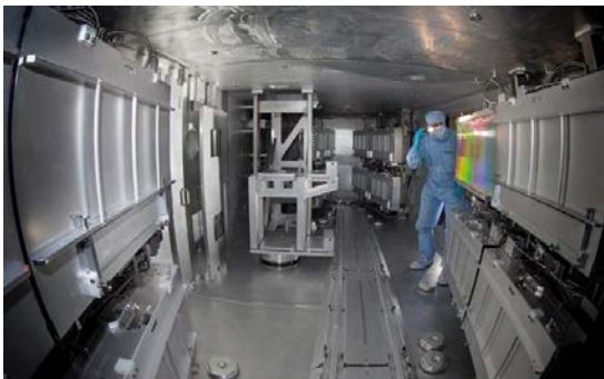
Figure 1. ARC compressor vessel uses 16 one meter-scale gratings to compress 4 ARC beamlets
