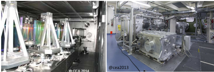
Figure 1 : PETAL in the LMJ Building with compression stage (left) and vacuum transport and focusing box (right).
